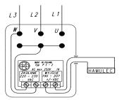
Supply circuit PS 2 forms a complete unit for direct installation. Provided with a four-terminal strip, it enables unhindered adaptation in every cooperating circuit. The circuit is adapted for supply from alternating current source of 220-230 VAC max. 250 VAC which after rectification and appropriate formation enables obtaining direct voltage of 190-207 VDC for brake supply.
