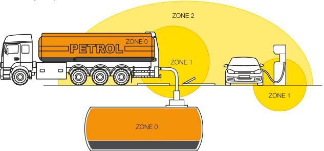
REMARK: Electric motors are not used in case of Zone 0 (gases) and Zone 20 (dusts).
