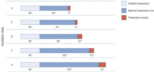
Insulation class F in an electric motor means that at ambient temperature of 40°C the temperature rise of the winding may be max. 105°C with the additional temperature margin of 10°C (under specified measuring conditions in accordance with the IEC 60034-1 standard).
