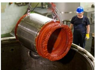
In order to enable supplying with power network available in sea ports the motors are designed for dual voltage and frequency.
