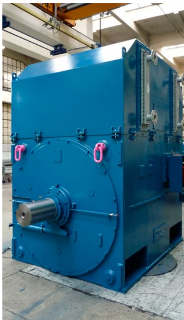
Output: 5600 kW, rated speed: 745 RPM, voltage: 10 500 V
