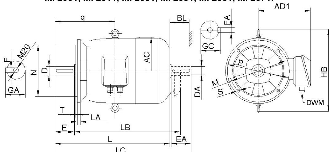
Typ **m(2)SKg** - forma wykonania:Type **m(2)SKg**-mounting arrangement:Typ **m(2)SKg** - Bauform:**IM 3001, IM 3011, IM 3031.**
