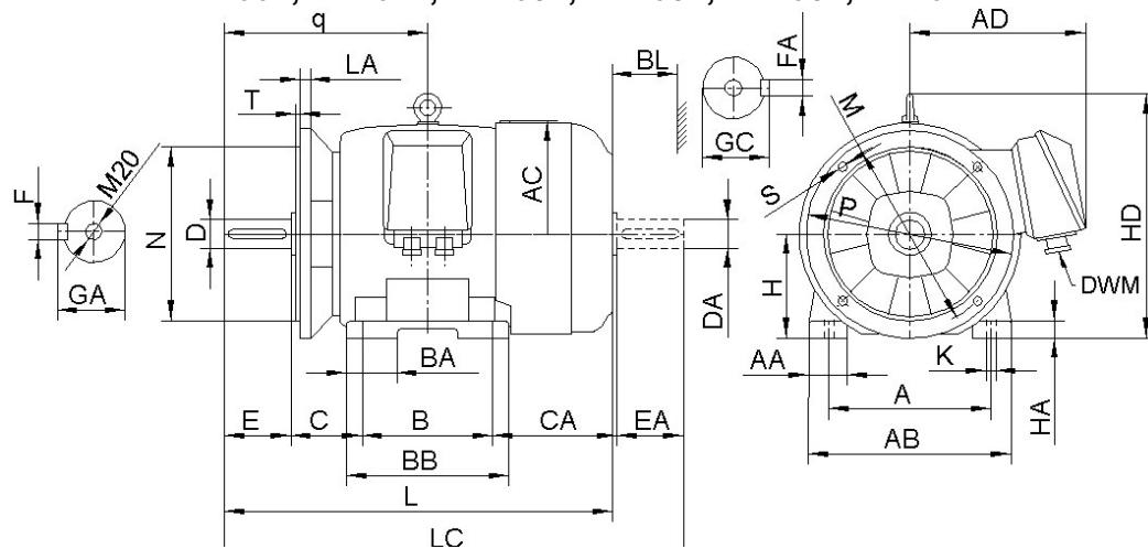
Typ **m(2)SLg** - forma wykonania:Type **m(2)SLg** - mounting arrangement:Typ **m(2)SLg** - Bauform:**IM 2001, IM 2011, IM 2031, IM 2051, IM 2061, IM 2071.**
