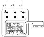
Supply circuit PS-1 forms a complete unit for direct installation. Provided with a four-terminal strip, it enables unhindered adaptation in every cooperating circuit. The circuit is adapted for supply from alternating current source of 380-400 VAC max. 420 VAC which after rectification and appropriate formation enables obtaining direct voltage of 170-180 VDC for brake supply.
