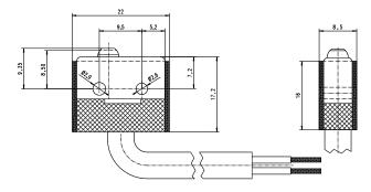
**Response monitoring microswitch**  $- \mathbf{KZ}$  - control of the state of brake (engaged, disengaged),
