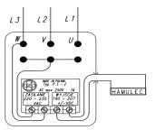
Supply circuit PS 2 forms a complete unit for direct installation. Provided with a four-terminal strip, it enables unhindered adaptation in every cooperating circuit. The circuit is adapted for supply from alternating current source of 220-230 VAC max. 250 VAC which after rectification and appropriate formation enables obtaining direct voltage of 190-207 VDC for brake supply.
