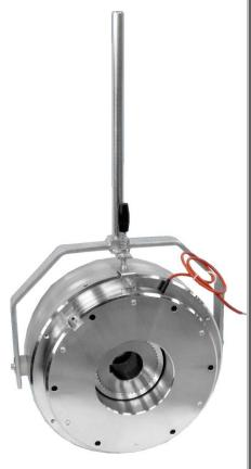
Brakes can be manufactured in variants suitable for various direct-current voltages: 104V, 180V which allows them to be supplied from standard alternating current sources, through appropriate rectifier.
